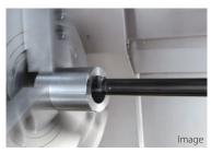
KAV-G20-10D / KAVH20-SCLCR09 CCMT09T304PP Overhang length: 140 mm (7D) / 200 mm (10D) Workpiece: SCM435
