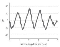
Cutting Conditions: Vc = 150 m/min, ap = 0.4 mm, f = 0.15 mm/rev Workpiece: SCM435 Overhang length 320 mm
