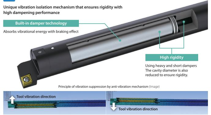
The damper vibrates late against the shank. Effective for vibration damping
