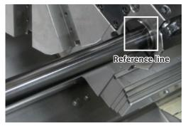
Adjusting the cutting edge position is easy by simply aligning the reference line between the shank and the sleeve.
