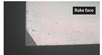
Flat land specifications to improve fracture resistance
