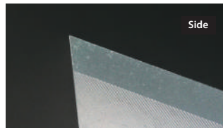
There is no land and a rake face is formed from the cutting edge Reduced impact forces when entering provides high-precision and stable machining ( \sim \phi 12 )
