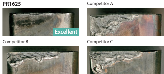
Cutting conditions: V_c = 140 m/min, f = 0.12 mm/rev, Insert width 3 mm Workpiece: SCM440 with 16 Slots External Grooving (Heavy Interruption)
